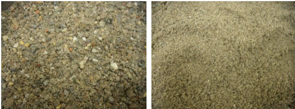
Figure 4 Left: Crushed concrete debris < 4 mm; Right: crushed concrete debris < 1 mm
