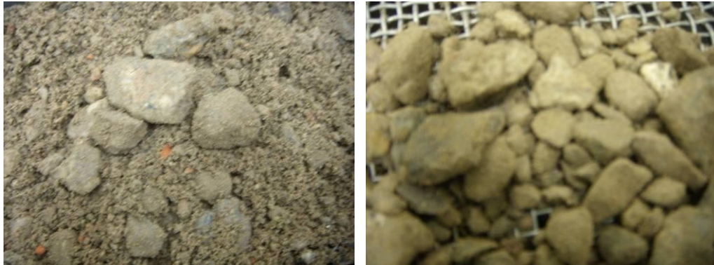
Figure 3 Left: Concrete rubble (0-20 mm); Right: sieve residue concrete rubble larger than 4 mm
