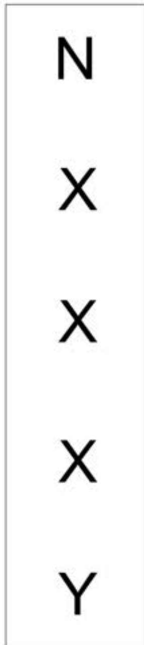
Figure 16.47 Type I motorway gantry label.
