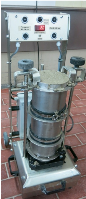
Figure 3: Compactor with clamped cylindrical mould filled with concrete
