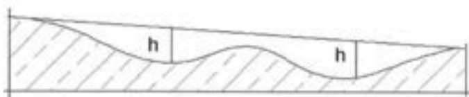
Figure 9.2: Flatness measurements with a four-metre straightedge on a concrete surface
