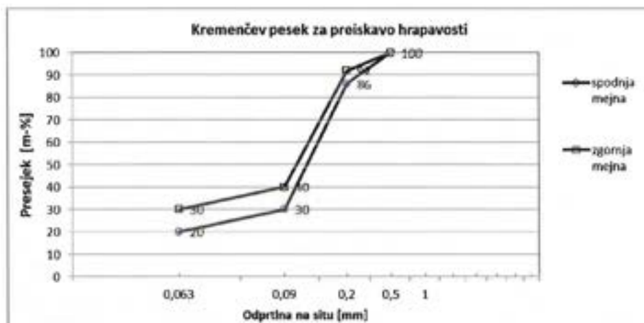
Figure 9.1: Granular structure of quartz sand for the test of the roughness of a concrete surface
